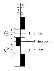
Fixing point in the range  $0^{\circ}$  ...  $270^{\circ}$  freely selectable
